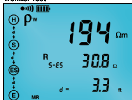
The Wenner test displays test lead connection, soil resistivity ( \rho ) test results, electrode spacing and resistance.
