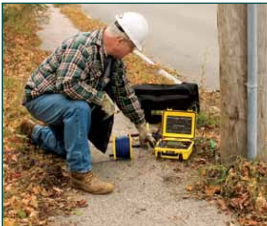
The Model 6470-B quickly checks ground rod resistance with its Connect – Press – Read approach.
