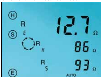
The 3-Point Fall-of-Potential test displays test lead connection, grounding rod resistance and test electrode resistances.
