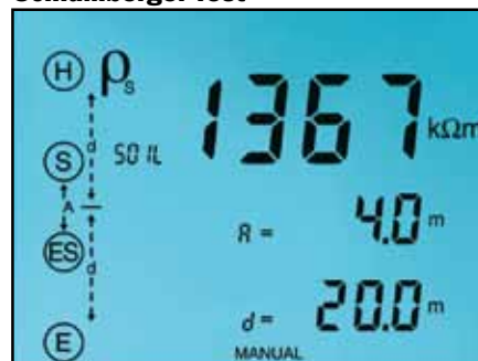
The Schlumberger test displays test lead connection, soil resistivity ( \rho ) test results and electrode spacing.
