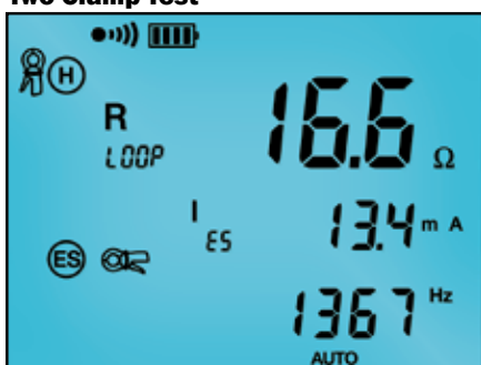
The 2 Clamp method displays clamp connection resistance, test current and frequency.
