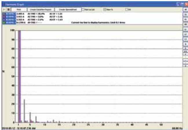
Display all harmonics from 1 st to 50 th in bargraph form for voltage, current and power.
