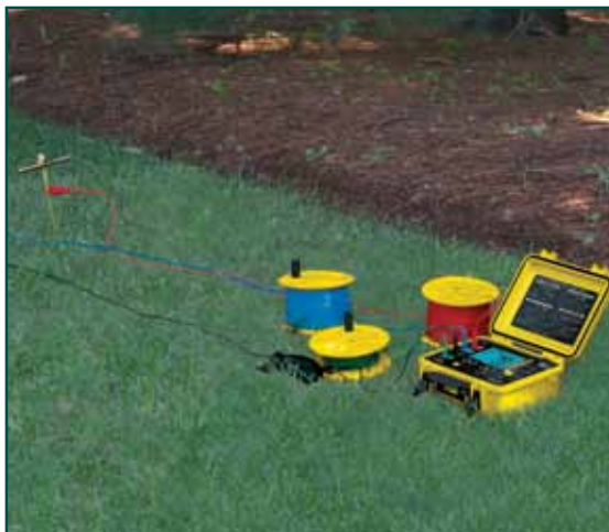
The Model 6472 performs an automated way to measure the value of the earth/ground using the Fall-of-Potential method and storing measurements.
