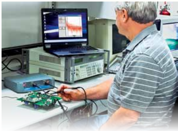
The MTX 1052-PC, MTX 1054-PC and MTX 162 can be connected directly to a PC via a USB or Ethernet interface with PC software. WiFi versions allow wireless Ethernet communication.
